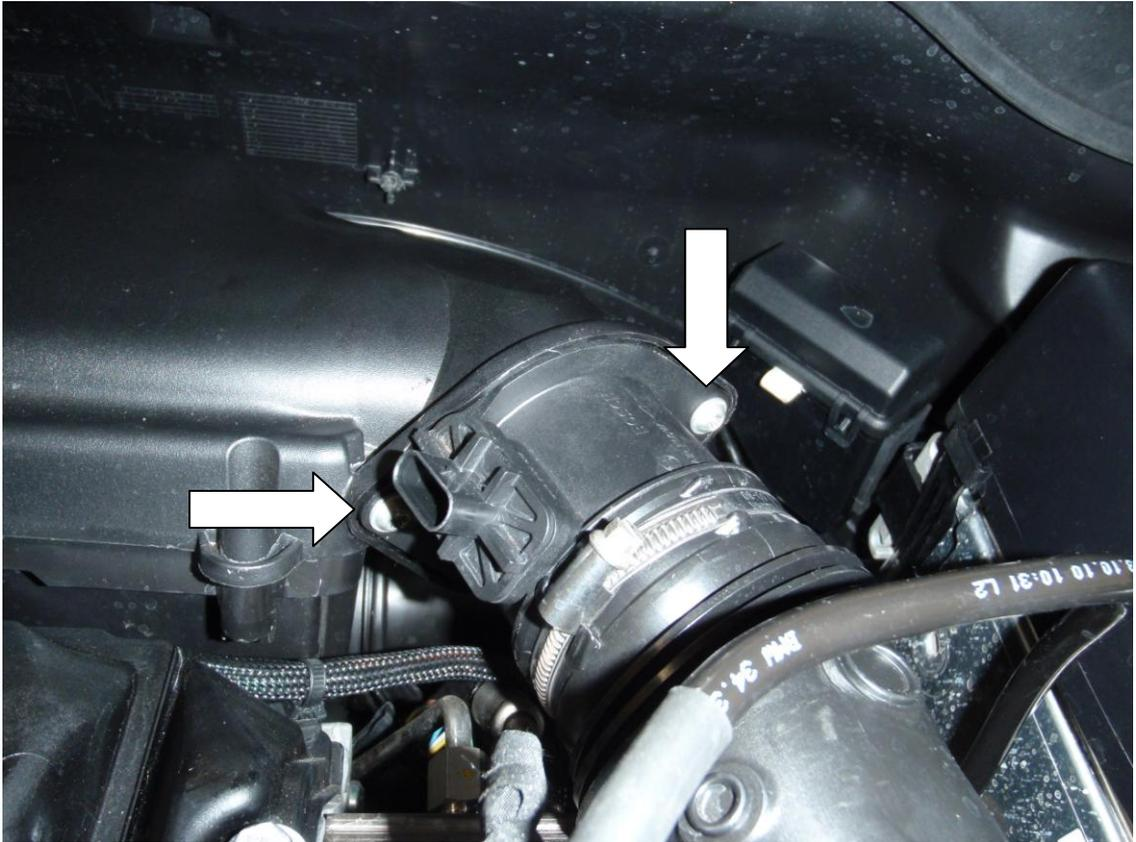
2. Undo the T25 Torx bolt holding the air filter down.
