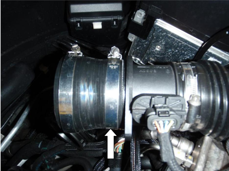
6. Fit the air filter to one end of the alloy pipe, and then the alloy pipe to the reducing silicon hose. Then using the self taper provided, screw that into the slam panel, tightening the 2 hose clamps.
