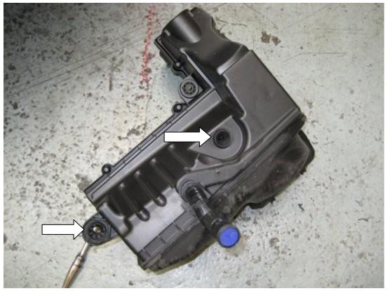
7. Remove the stock plastic scoop from the rear of the slam panel, then fit the new Forge air scoop reusing the stock screws.
