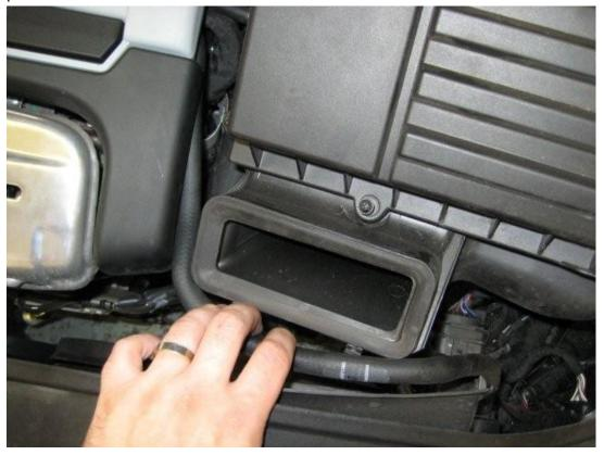
6. Grab each side of the airbox and pull sharply upwards to release it from the two rubber locating lugs on the underside, then remove it from the car. Locations of the rubber lugs shown below.
