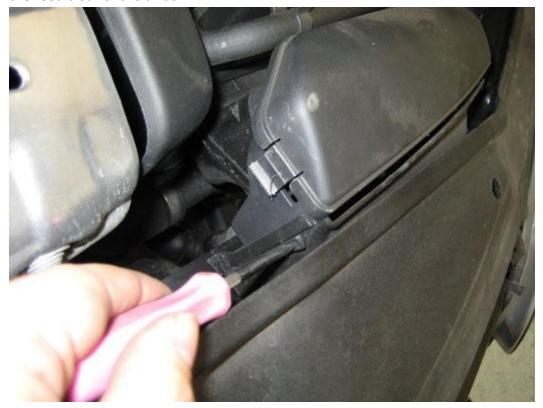
5. Push the water pipe down the front edge of the airbox so that you have clearance to pull the airbox free.
