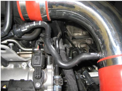
9. Fit the remaining silicon 76-70mm reducer to the airfilter, then fit to the air scoop and intake pipework, with jubilee clips and tighten all jubilee clips fully when all in place. Lubricating the joiners with silicon spray will help with fitting.
